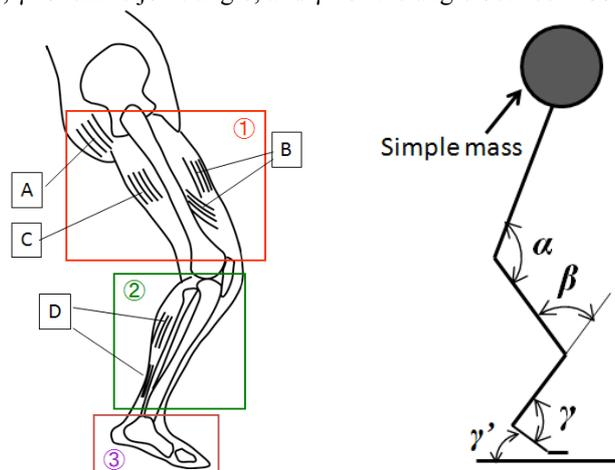
Fig. 1 A 2D model of a lower limb and definition of the joint angles.
