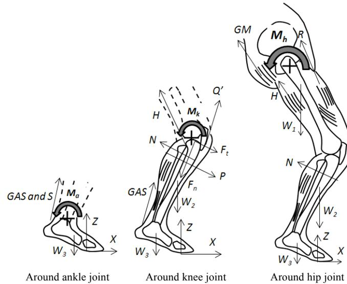
**Fig. 2** Forces for calculating the moment equilibrium condition around each joint.
